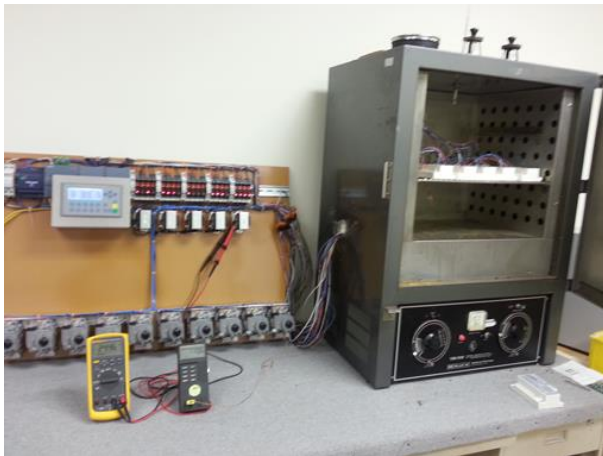
Frymaster 9X life test set-up and temperature chamber
